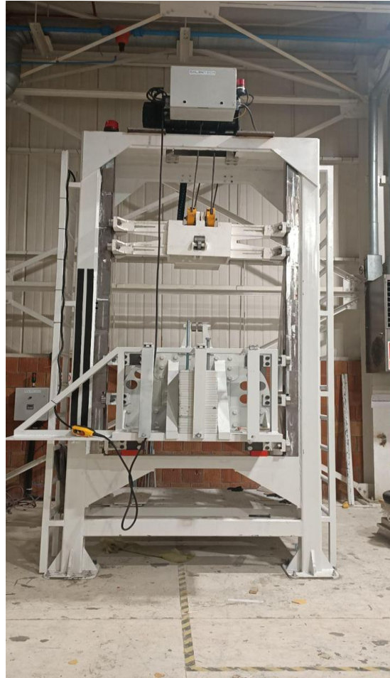
Drop Test Unit
